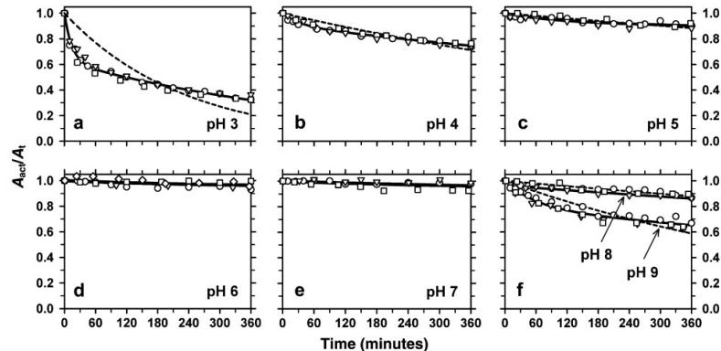
Fig. 1. Fraction of residual activity ( $A_{act}/A_t$ ) as a function of time for laccase incubated at various pHs. Experimental conditions: 25 °C with  $A_t = 2.8 \text{ U mL}^{-1}$ . Different symbols are data points arising from independent experiments. Solid and dashed curves were generated by curve-fitting Eqs. (2) and (3), respectively, to activity data. Equation parameters are presented in Table 1.
