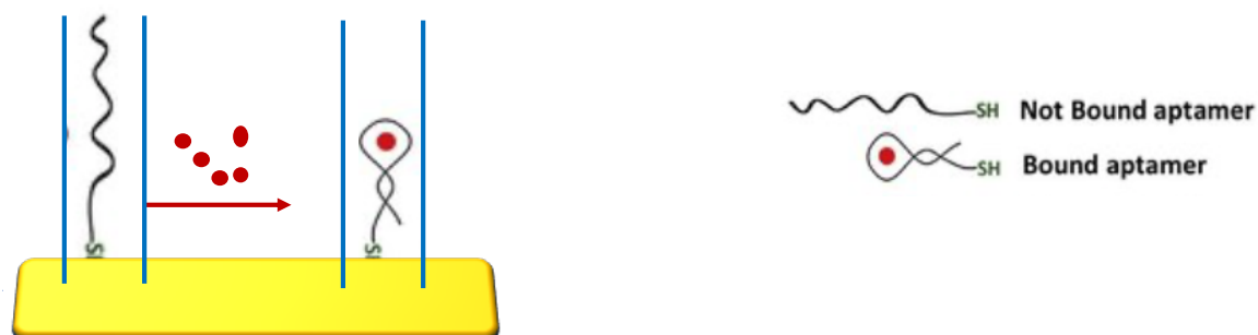
Figure: Aptamers immobilization via improved ESI-thiol-linker and development of reliable aptasensor for troponine
